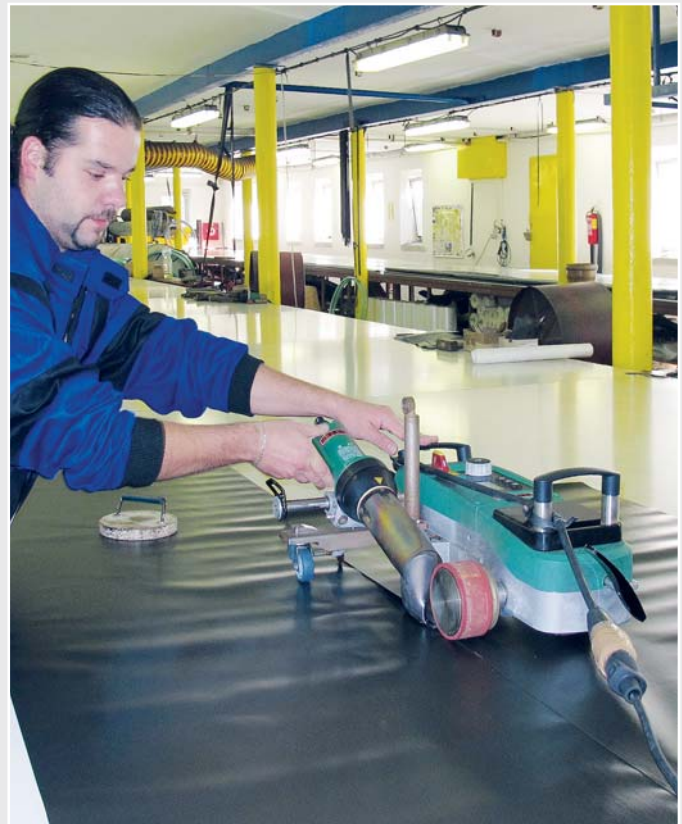
Simple guidance of the VARIANT T1 during the welding process.
