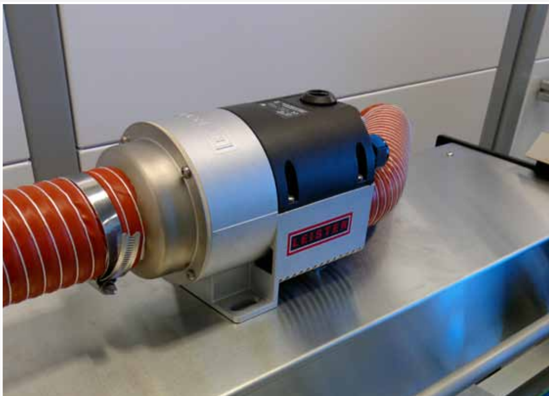
An air heater LHS 60 S from Leister supplies the drying module with the required heat at sufficient air throughput. (photo: Tronrud)
