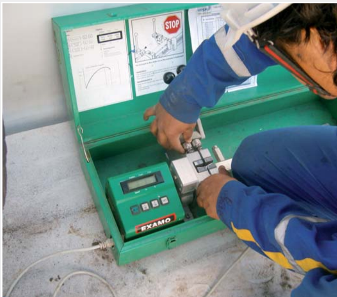
The tensile tester EXAMO for checking the relevant welding parameters.
