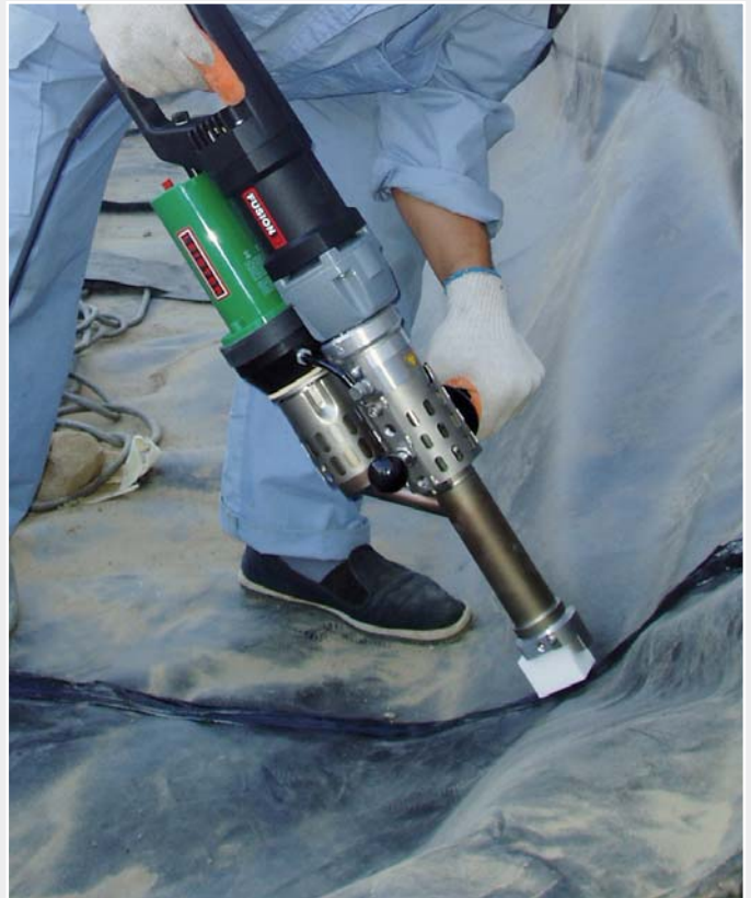
The hand extruder FUSION 3 for upright extrusion welding without strain
