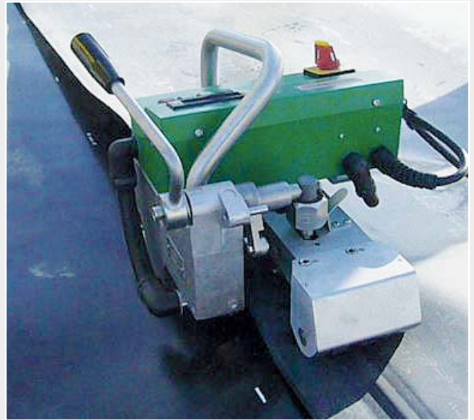
The ASTRO welds the HD-PE sealing tracks at a speed of up to 5 m/min.
