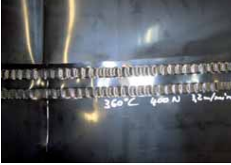
Flawless test welding with the combi-wedge welding machine TWINNY T.
