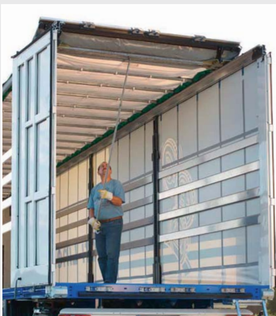
Tarpaulin bows for fixed and sliding rooftops of lorries (Pictures: Krone).
