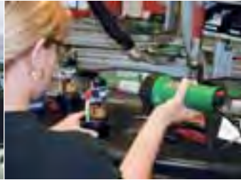
Shrinking a solder sleeve with TRIAC PID.
