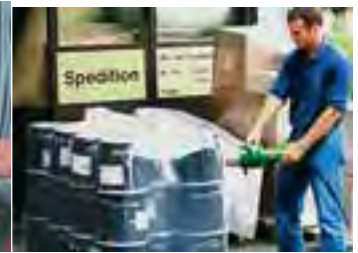
Flameless shrink-wrapping of pallets and bulky goods with the FORTE S3. This allows work to be carried out in closed spaces.
