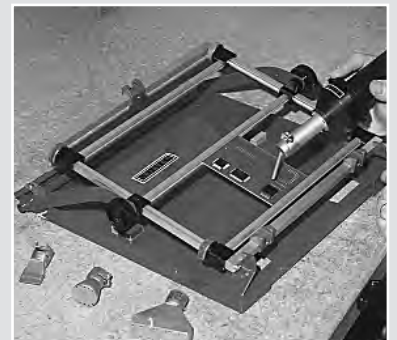
After positioning the SMD component it is then soldered in seconds.
