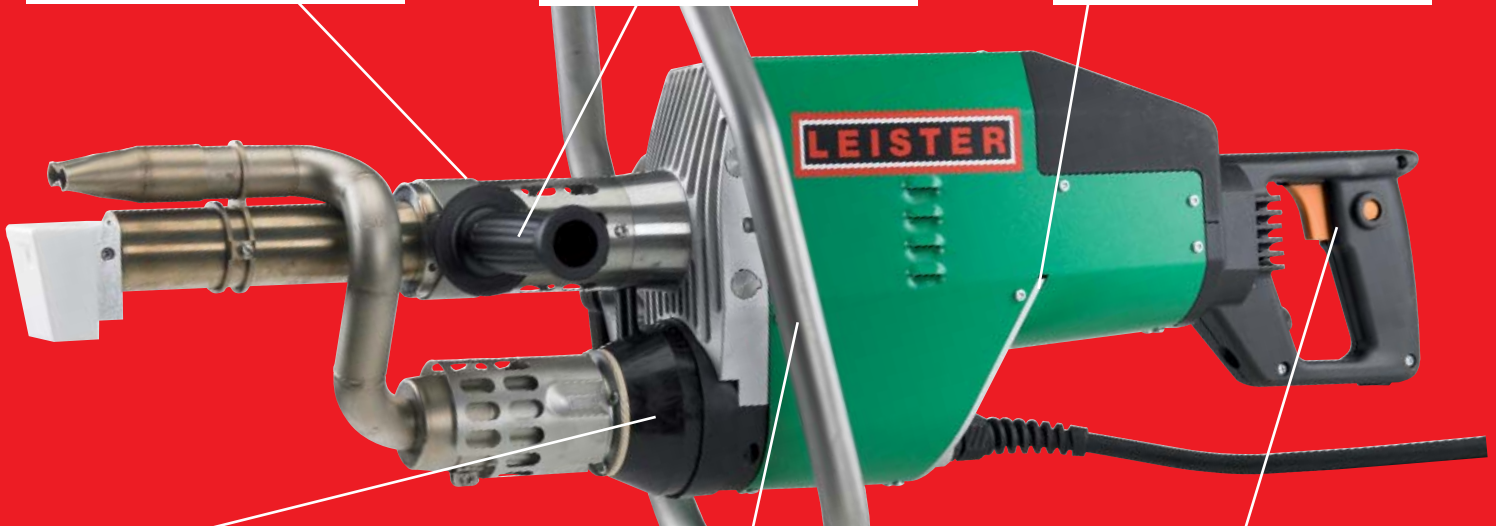
Symmetrical handle fixation mountable left and right
